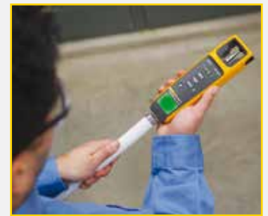
Pin continuity test: Tests if filaments have continuity
