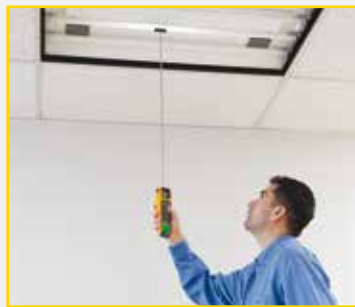
Lamp test: Test bulb without removing from fixture
