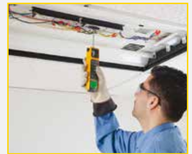
Ballast test: Easily determine if ballast is working
