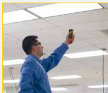
Ballast-type test: Determine if ballast is electronic or magnetic without taking fixture apart – identify energy wasting ballasts
