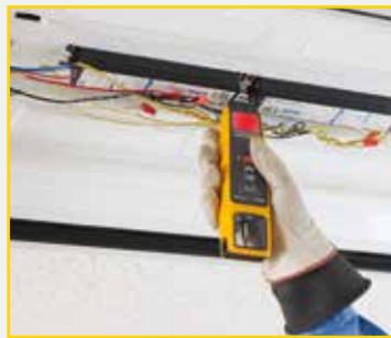
Non-contact voltage test: Quickly check for voltage presence
